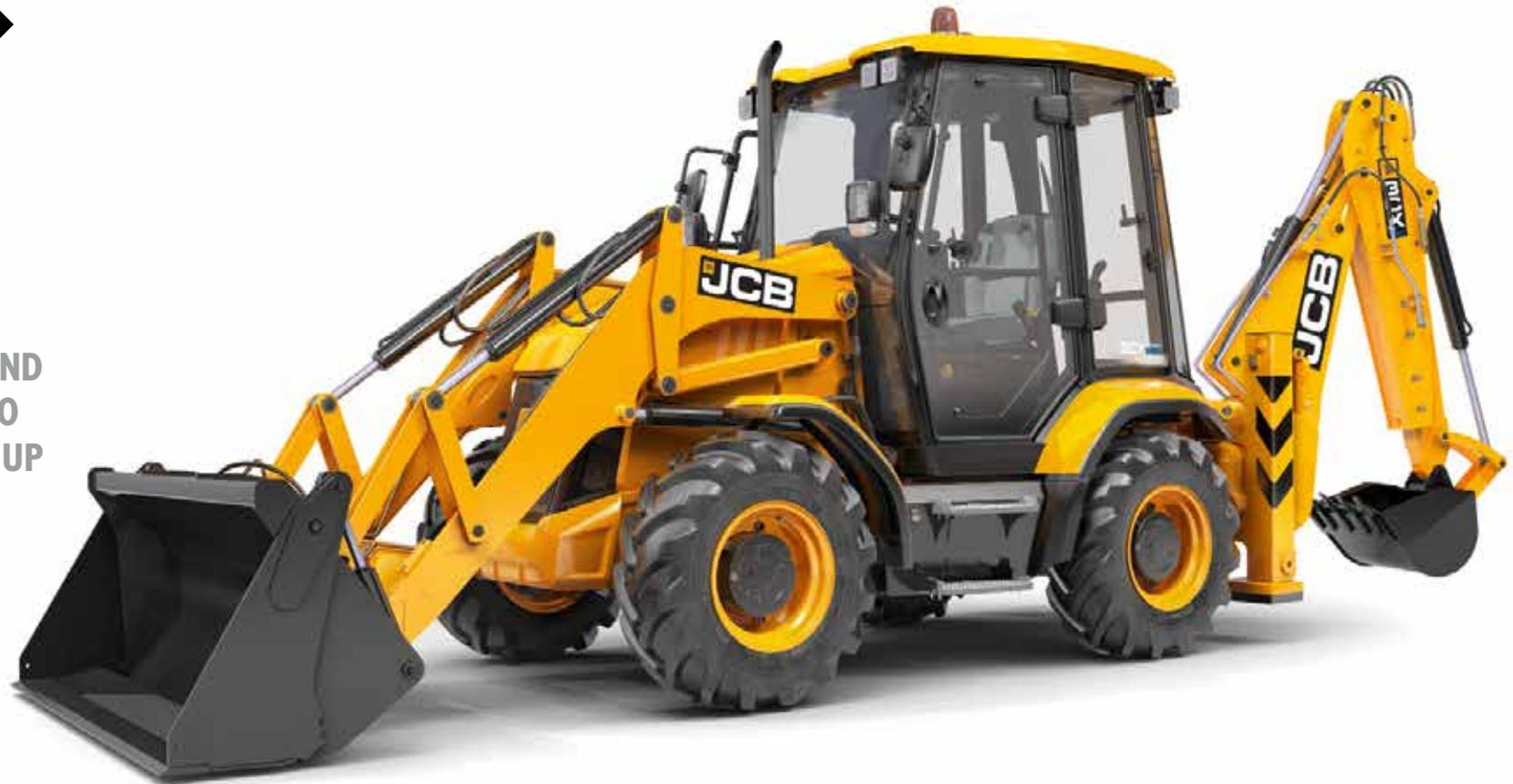
A 3-in-1 machine, the 3CX Compact can be a compact excavator and wheel loader, with skid steer attachment versatility.
