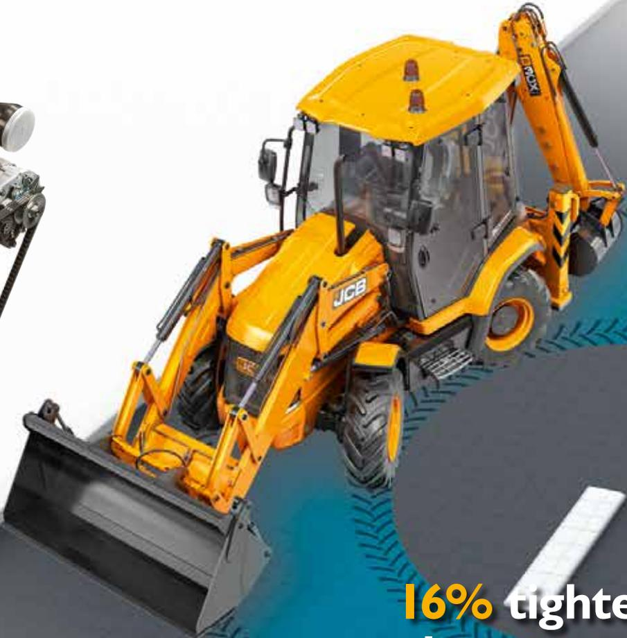
An impressive 5.8 metre turning circle (with applied brakes) allows the machine to turn a full 180 degrees in a single carriageway.
