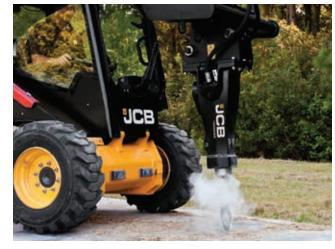
Properly matched tool and piston ensures maximum energy transfer for the material being broken.
