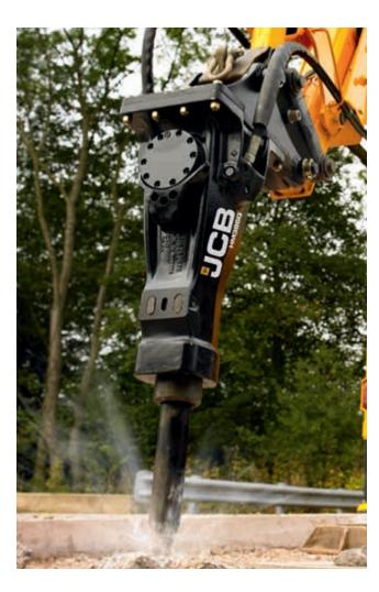
The sealed-for-life accumulator is maintenance-free for minimum downtime, and only needs recharging during a full rebuild. Diaphragm support reduces wear.
